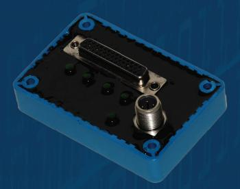
This module is designed for more complex strain data collection. For simple strain gauge configurations use the 12-Cannel Strain to CAN Module.
